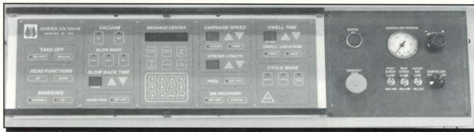
Operator's control panel and air controls
