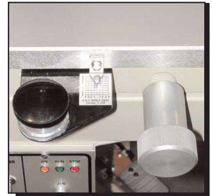
Registration Multi-directional micro-adjustable printing table with witness grids for fast and easy registration
